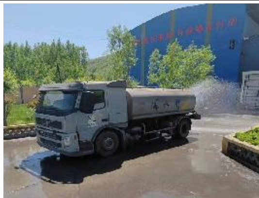
洒水车洒水抑尘
